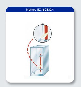
A 60 cm long piece of cable is exposed to a flame for 60 seconds. The cable must not ignite.
