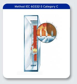
A cable bundle is exposed to a line of flames for 20 minutes in a 4 meter high cabinet. Approximately one meter above the flames the cable bundle must extinguish itself with only a minimal production of smoke.
